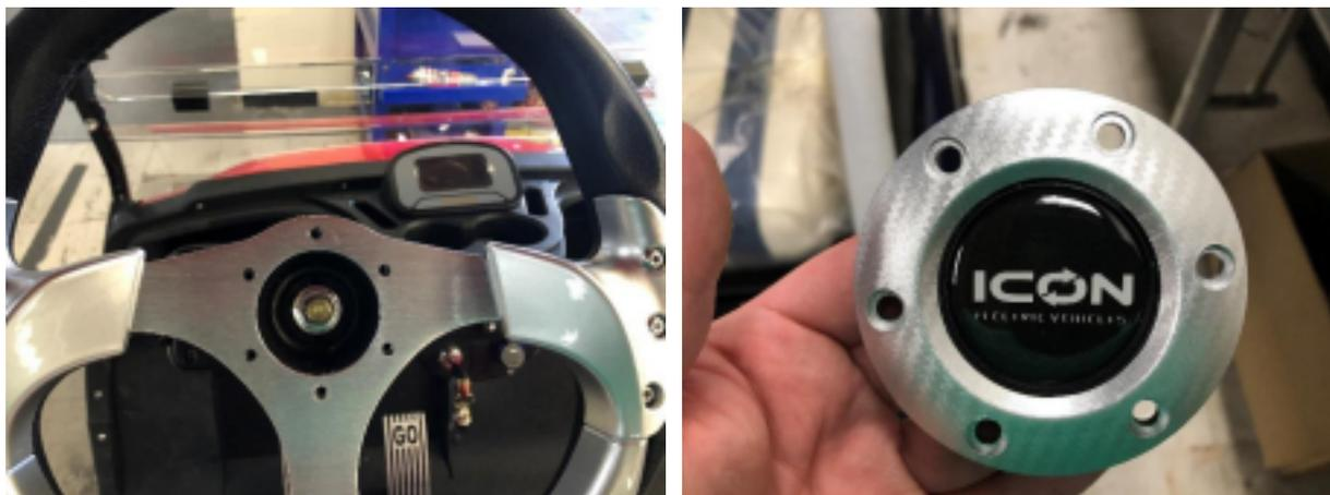
Pictured is the steering wheel with the trim ring and center cap removed
