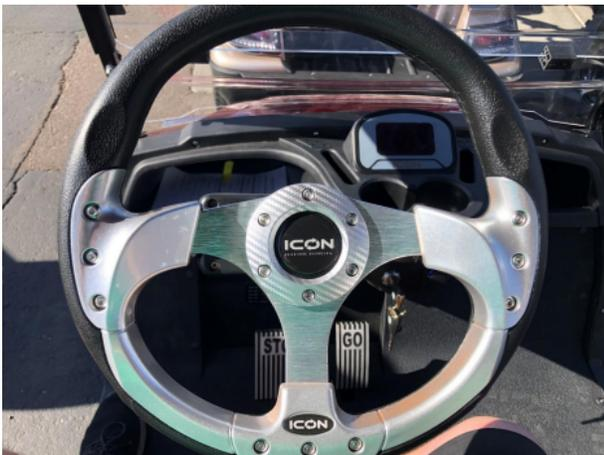
Once the 6 allen heads have been removed the steering wheel may be set aside
