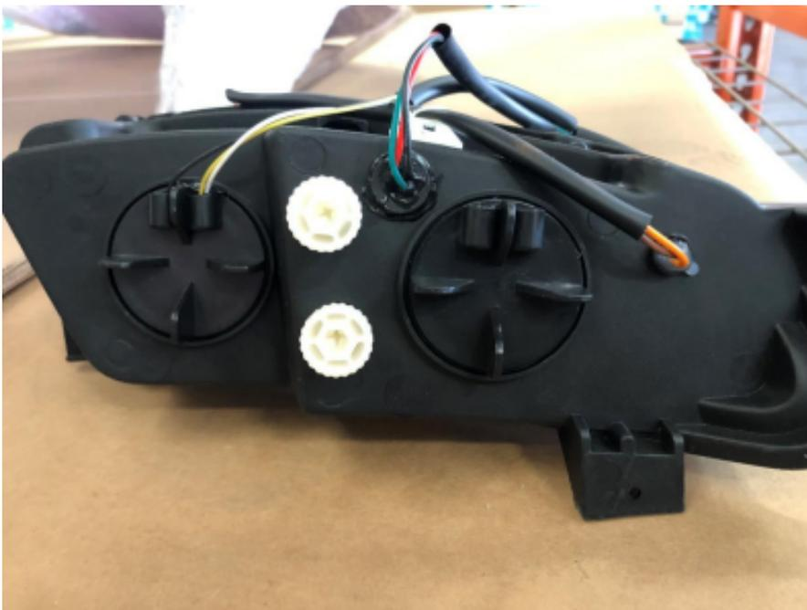
The knobs control up and down motion, but also control a telescoping motion. The farther the lights are telescoped out, the wider the light beams will get.
