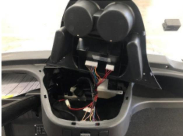
At this point you will now have access to the back of each headlight. You will need to reach in as far as you can to reach the knobs. It is a very tight fit and the knobs are snug. If you cannot get the knobs to turn you can try and use a very small set of channel locks to get a better grip on the knob to turn.
